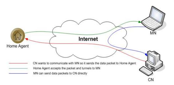
Figure 2.2: Mobile IP routing
