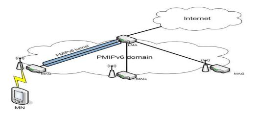
Figure 2.5: PMIPv6 domain basic configuration
