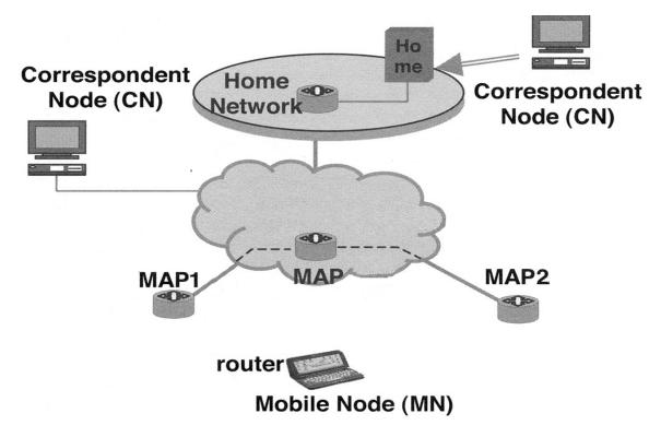
Figure 2.3: A typical HMIPv6 network [16]
