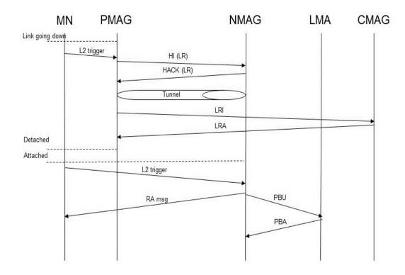
Figure 3.5: Call flow for O-PMIPv6 in topology 1
