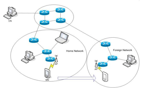
Figure 2.1: An example of a mobile node moving from one network to another
