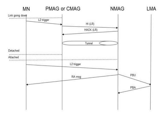
Figure 3.9: Call flow for O-PMIPv6 in topology 3
