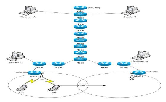
Figure 5.1: Default network topology used in the simulation
