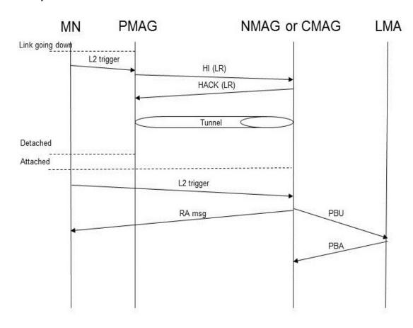
Figure 3.7: Call flow for O-PMIPv6 in topology 2
