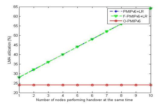
Figure 4.6: Number of nodes performing handoverys. LMA utilization
