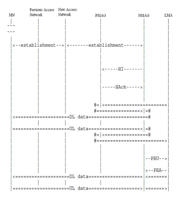
Figure 2.10: Reactive Fast Handover for PMIPv6 [2]
