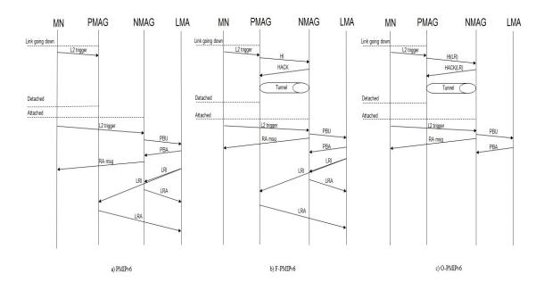
Figure 4.2: Signaling flow for mobility protocols with LR
