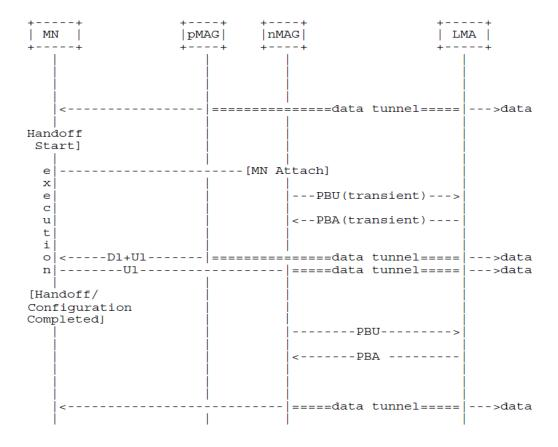
Figure 2.11: Transient Binding for PMIPv6 [22]
